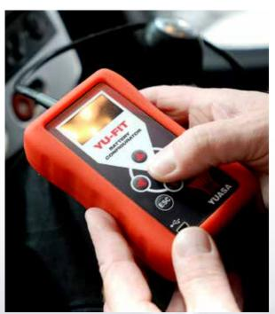
An increasing number of automotive manufacturers have introduced systems that now require a replacement battery to be correctly configured to the vehicle after installation.
